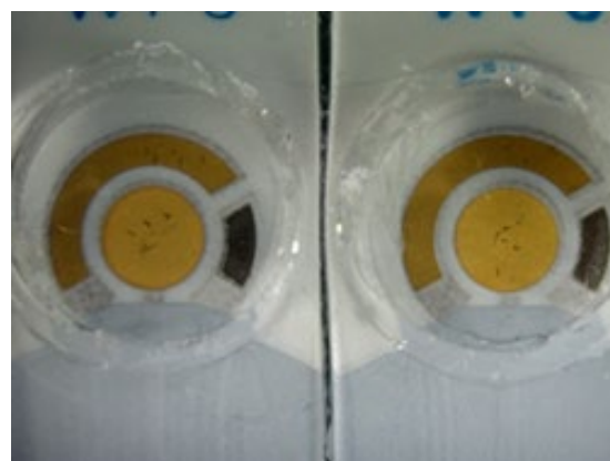
Figure 1: Electrode array with defined surface using PDMS
