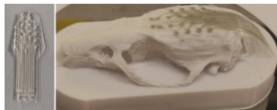
Figure 1: The multi-electrode implant on glass substrate and fitted on the skull
